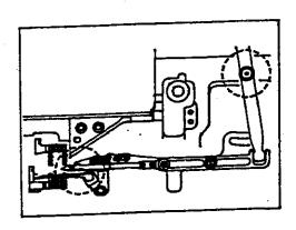
WHEN THE MOVABLE KNIFE MOVE TO 1.5m.m. FROM THE LEFT EDGE OF FEED DOG'S RIGHT COLUMN.
